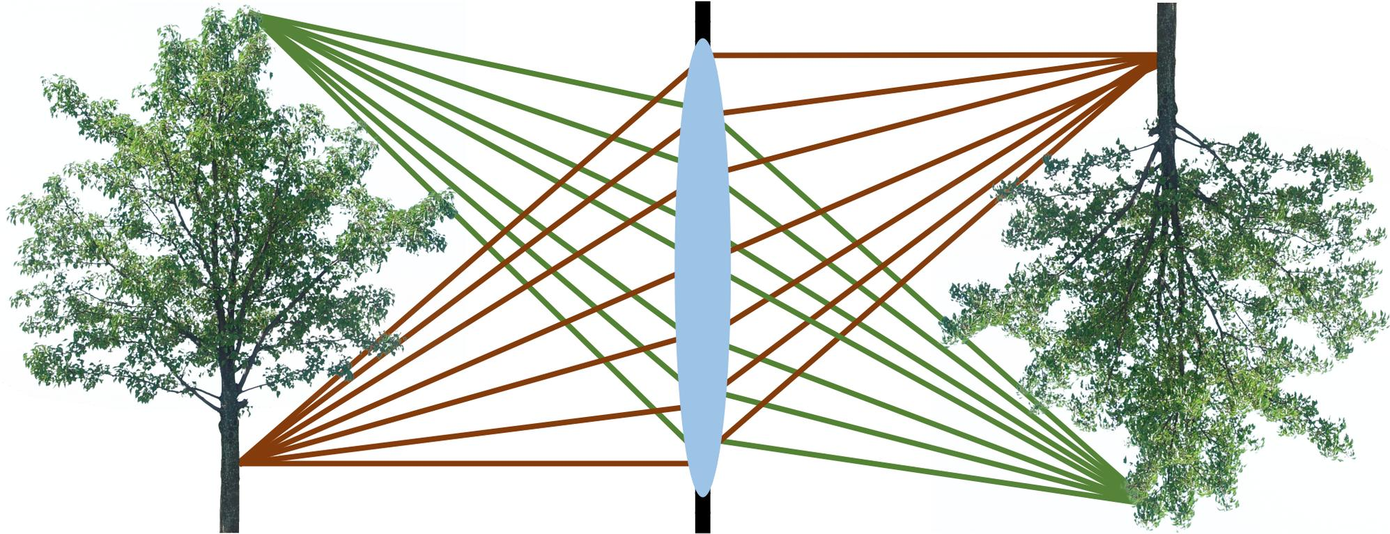
Central rays propagate in the same way for both models!
